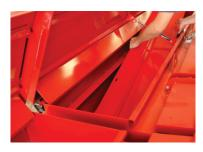
Hoppers. they have a system of moving parts that allow increase by 40% the capacity in cases where no fertilizer is used.
